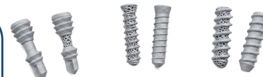
Figure 7: Version 2 CAD models after incorporation of lattice: Self-tapping (left), Buttress (middle), Cylinder (right).
