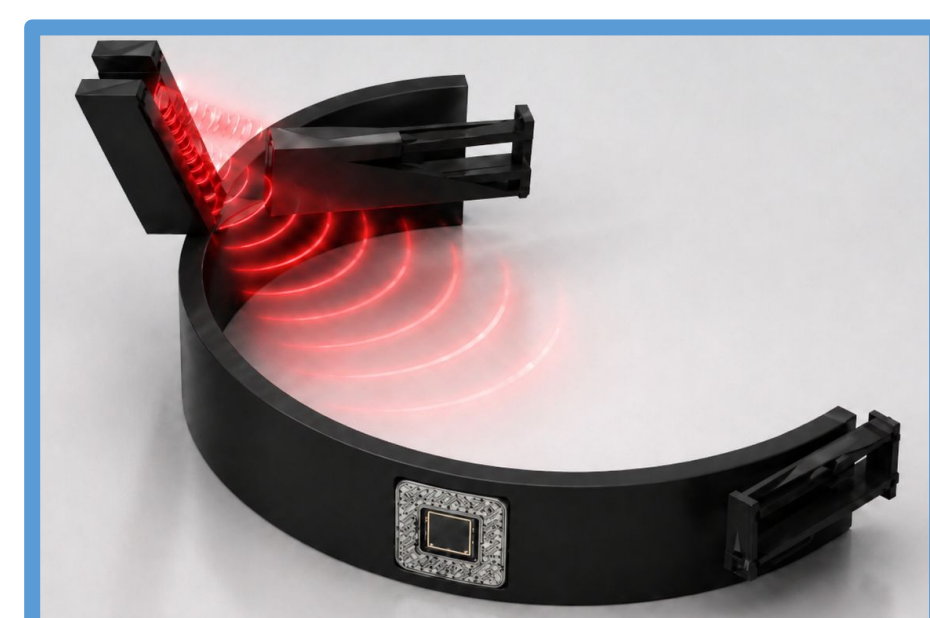
Figure 6: Old concept of a 3D printed holding device made of TPU to hold the photodiode and LED in the ideal position.
