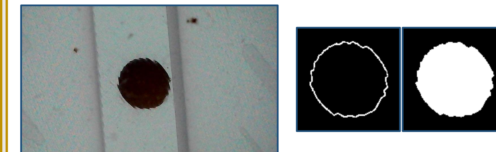
Fig 9. Real-time raw camera image of bead phantom in channel (left) & image processing output of binary masks (right), which was accurately classified as "good".
